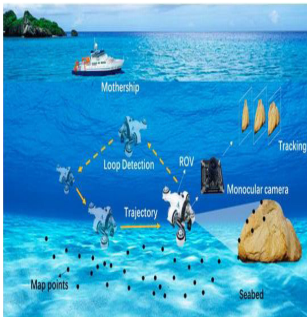
Fig. 3. Path-tracking and localization of an underwater robot. https://www.mdpi.com/1424-8220/22/13/4657 .
