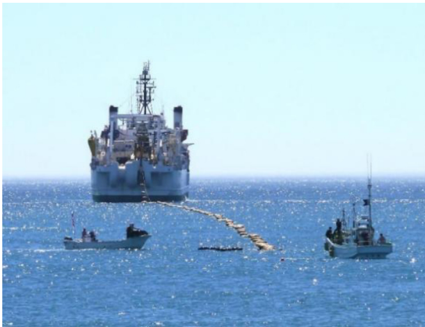
Fig. 15. Cable laying ship deploying subsea cable in the Pacific Ocean. https://newatlas.com/one-big-question-faster-cable/45430/ .
