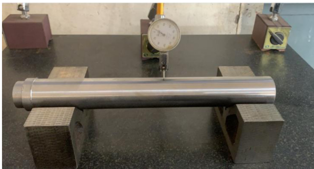
Fig. 2. Measuring RE with a dial gauge.
