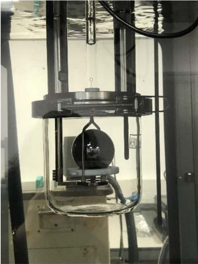
Fig. 5. Silicon sphere and holder.
