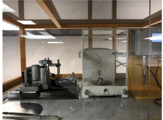
Fig. 4. Automatic mass loading system.
