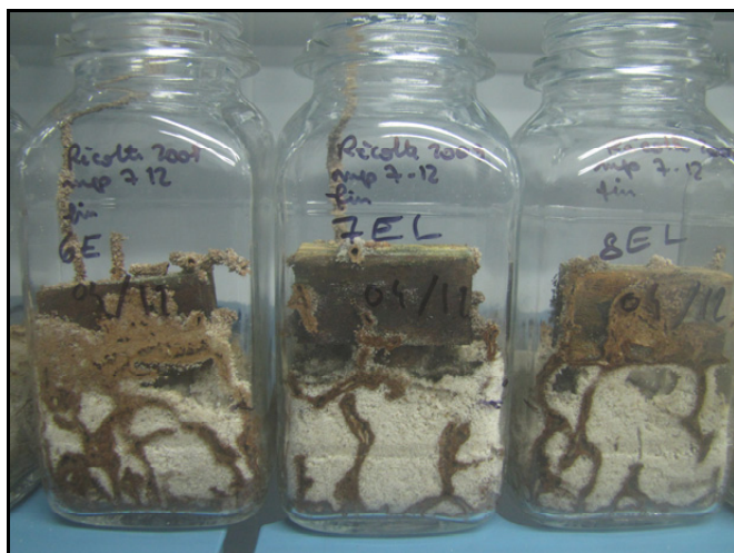
Fig. 7. Culture flasks (test device) with termites.
