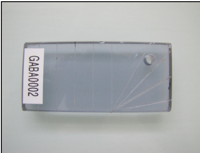
Fig. 1. Test gauge for wood sample selection ( \pm 1 mm, \pm 1^\circ ).
