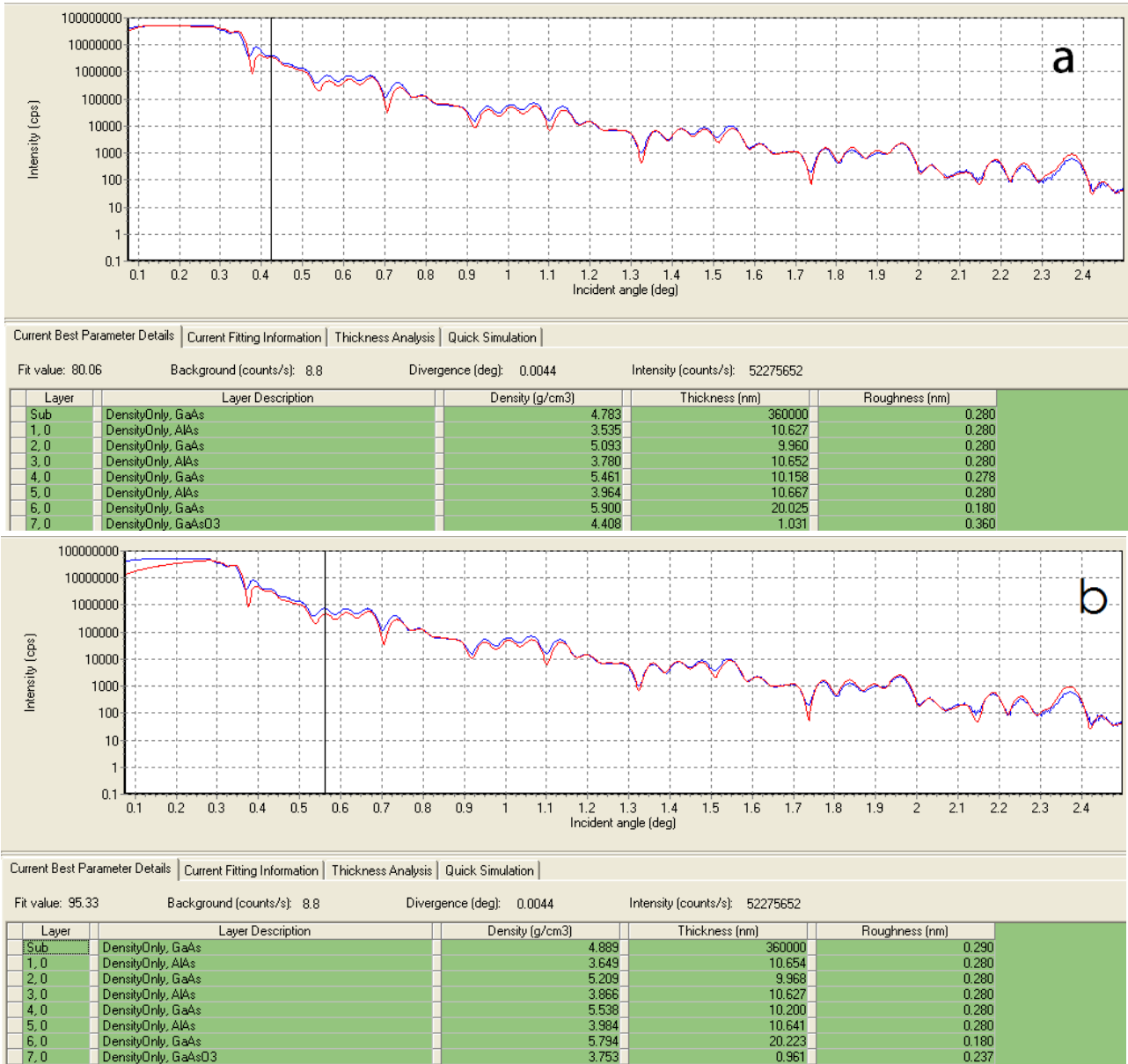
Fig. 2. The simulation results of superlattice determined by GIXRR.
