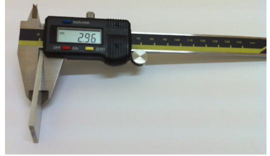
Fig. 2. Measurement of test sample dimensions by calliper.
