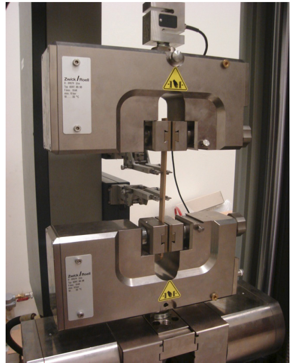
Fig. 2. The photo during tests. Including sample, grips, extensometer and force transducer.
