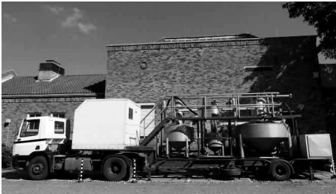
Fig. 1. Proving tanks 500, 1500 and 4000 L on trailer.
