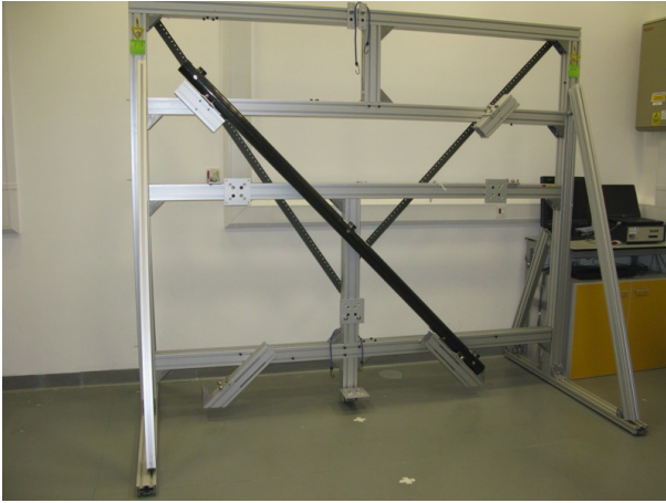
Fig. 3. B89.4.19 artefact and support rig.
