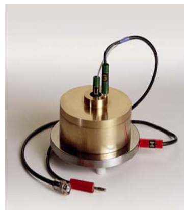
Fig. 3. (Color online) Solid test cell.
