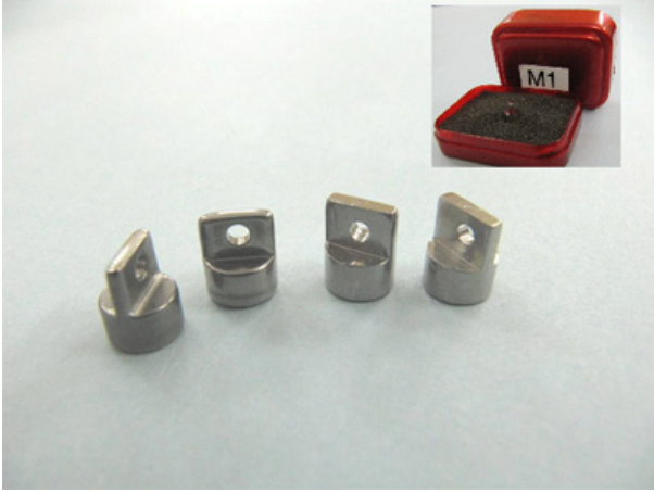
Fig. 2. Set of polished mass samples. Inset shows the standard packaging provided.
