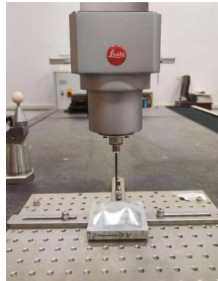
Fig. 8. Free-form surface part measurement using the coordinate measuring machine.
